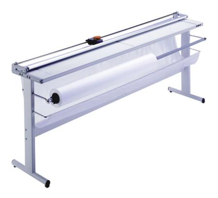
Manual cutter ideal for cutting drawings, photographs, posters etc. A choice of several different cutting widths. Smooth running blade carriage. Rotary blade in hardened steel. Fixed blade in inox. Sheet press made of transparent plastic. Available with or without stand and retrieval tray for trimmings. Metallic components epoxy powder coated, colour grey RAL 7035. Accessory: roll-holder and lamp over cutting area.
